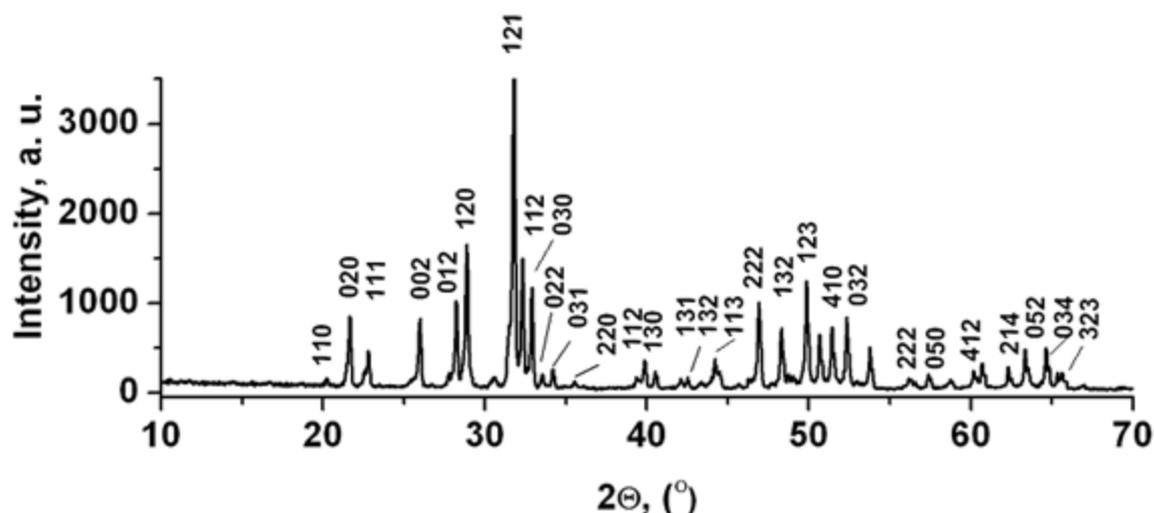
Fig. 1. The X-ray diffraction patterns of  $\text{Ca}_2\text{Y}_{6.4}\text{Eu}_{1.6}\text{Si}_6\text{O}_{26.5}$
